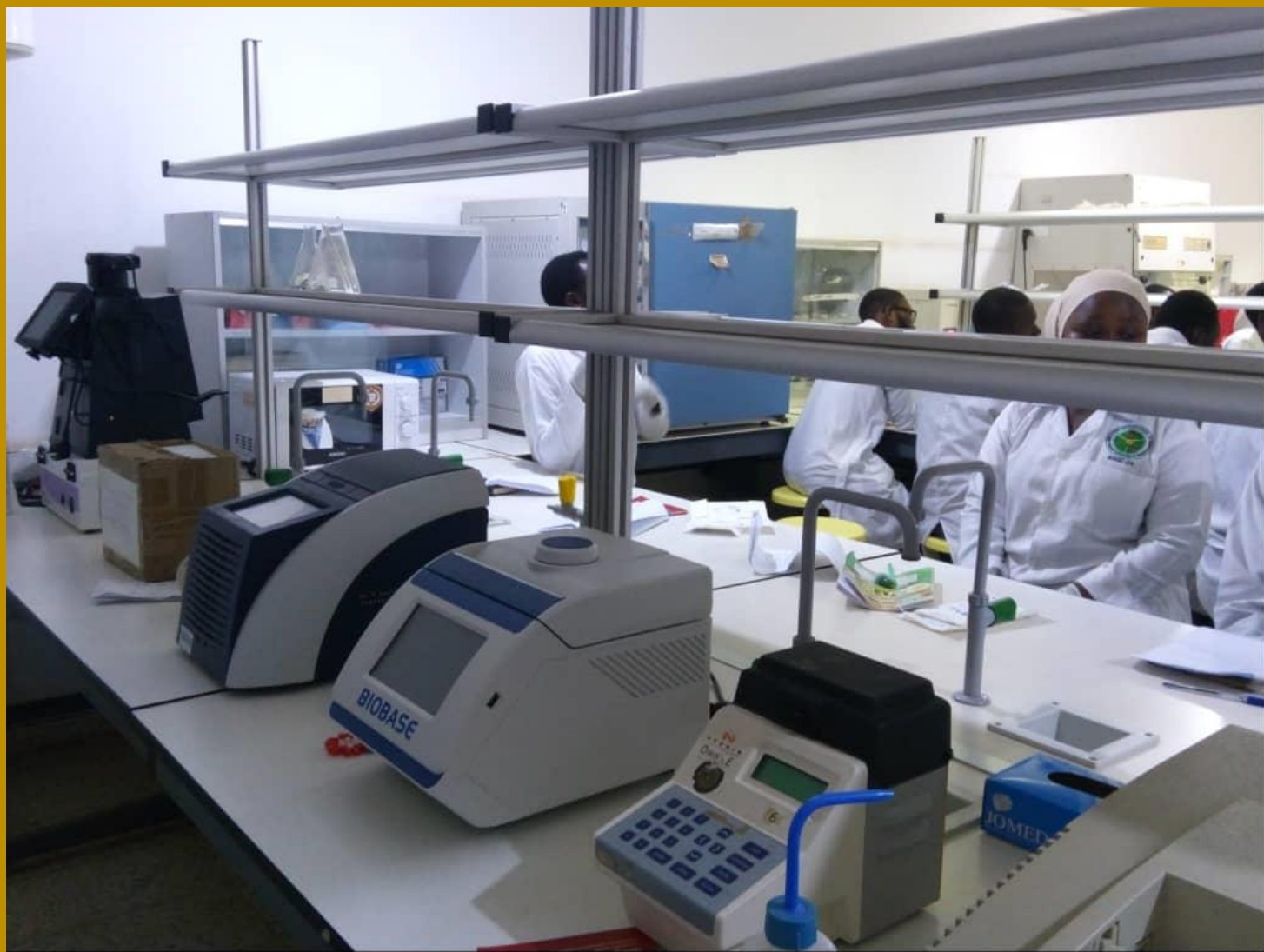
Plate 8: A cross-sectional display of molecular biology equipment – Thermal Cyclers, UV chamber, gel documentation unit, etc.
